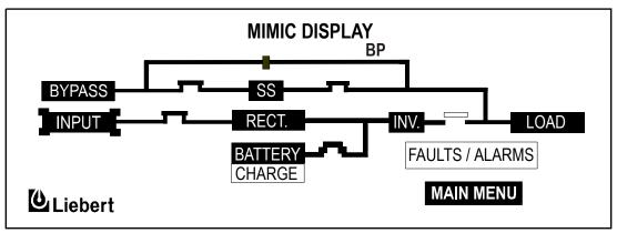
In this example, the load is receiving power through the bypass switch. Notice that the input power source is available and the battery is being charged.
